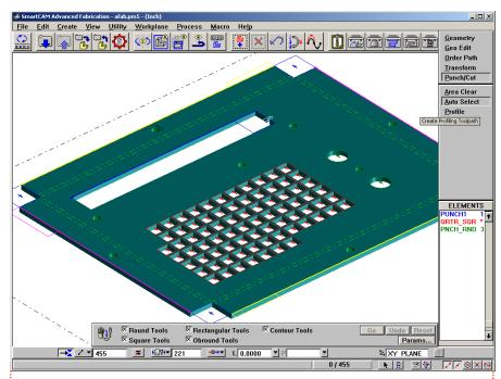
SmartCAM Advanced Fabrication Optimized punch hits for power supply front panel
