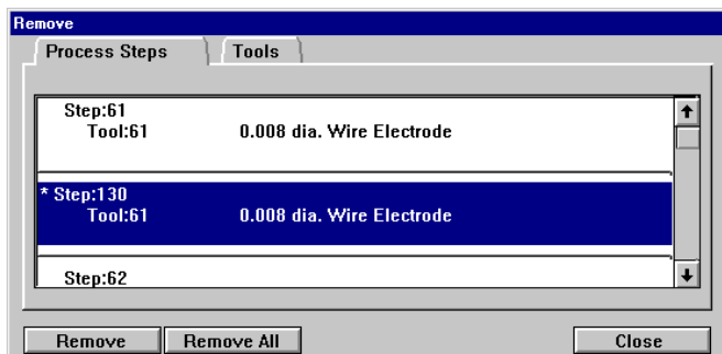
Figure 3-28 Use the Remove dialog box to specify steps or tools to remove from the Job Operation Planner.
